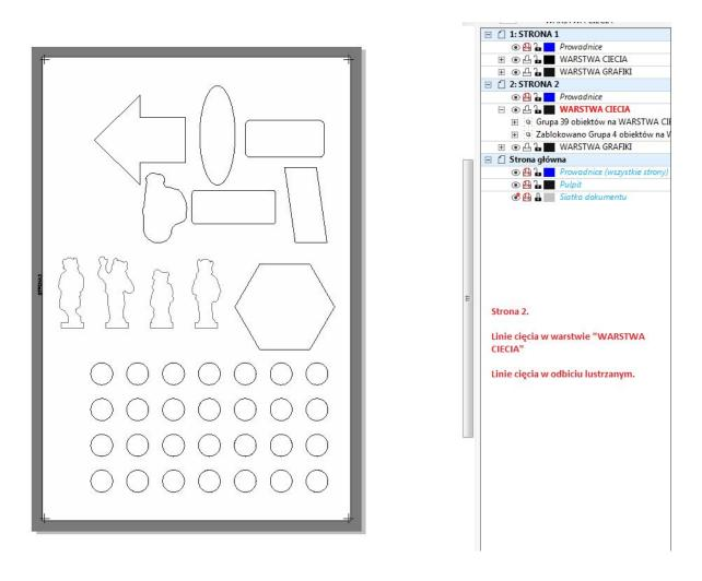
Place the token shapes on the chosen template. Place the cut lines in the "Cutting LINE" layer. Do not remove any marks on the sample sheet in the white field.
